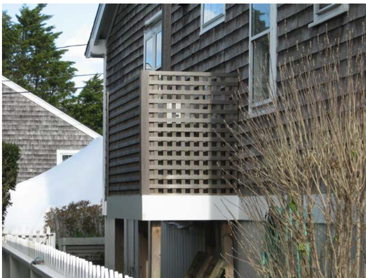
YES: Lattice panels, slats or landscaping are recommended to screen mechanical units from view.
